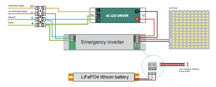
When luminaire is permanently connected to mains supply, allow the luminaire to fully charge for 16 hours conduct following tests once the battery has fully charged
