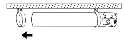
③ After the light sitting in the right position, fix the screws on the sides Turn on the power to ensure the light is working properly
