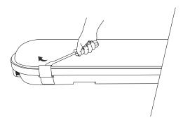
4. Loosen the cable gland nd insert the power cable through the cable gland.
