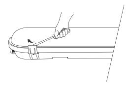
4. Loosen the cable gland and insert the power cable through the cable gland.
