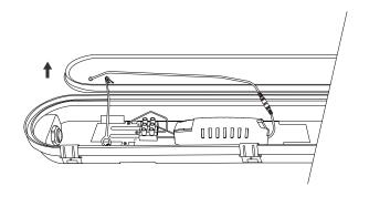
5. Connect the power cable o the driver and tighten the cable gland.
