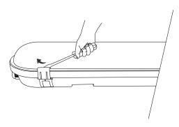
4. Loosen the cable gland nd insert the power cable through the cable gland.
