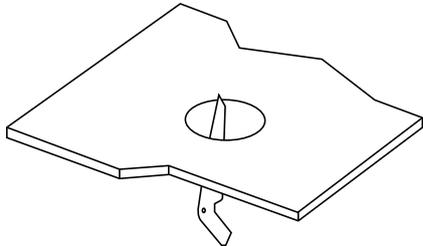
2. Use screw-driver to open the driver terminal cover, feed the main AC wire L. N. in terminal block respectively, then fix the cover back.
