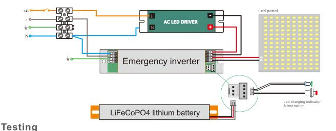
When luminaire is permanently connected to mains supply, allow the luminaire to fully charge for 24 hours. Conduct following tests once the battery has fully charged:
