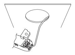
4. Make sure the downlight fixed tightly in ceiling, turn on the power.
